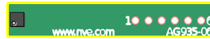
AG935-06: DFN6 connection board for -10E suffix sensors. (1.57" x 0.25" / 40 mm x 6 mm; actual size).
