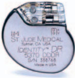
▲ St. Jude Medical, a pacemaker manufacturer, is using NVE Corporation's giant magnetoresistive (GMR) sensors, which are highly stable and sensitive magnetic sensors, to replace the reeds of conventional pacemakers. The GMR sensors are an order of magnitude more sensitive than the reed, and they are solid-state devices, not mechanical.
